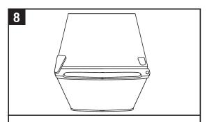
Check that the door is aligned horizontally and vertically and that the seals are closed on all sides before finally tightening the upper hinge. Re-adjust the leveling feet.
