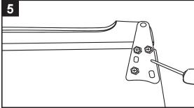
Screw the three screws to install the top bracket on top right side of appliance. Slide the appliance door back on to the top hinge. Making sure it's face up. Then replace the "plastic cover" on the top bracket by clicking back into position of door hinge.
