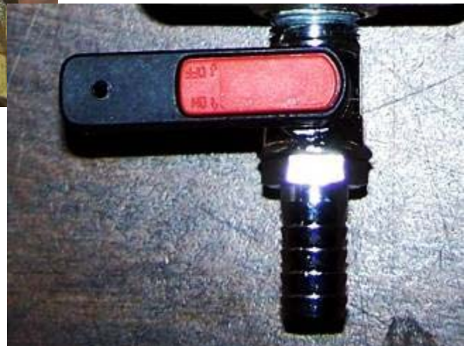
Below: One type of secondary cut off valve in the "OFF" or "Closed" position. In this position, no air is flowing to the coupler. The lever would be down for the "ON" or "Open" setting. Open allows air to flow to the coupler.
