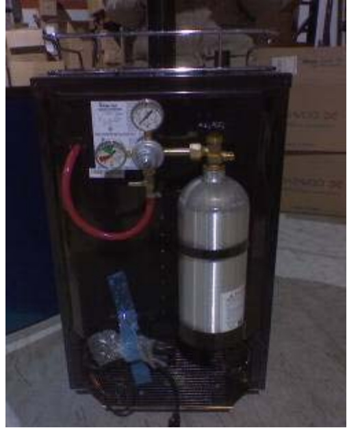
View of the rear of the unit with the cylinder bracket, CO2 cylinder, regulator, and air hose.
