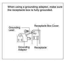
NOTE: THE CANADIAN ELECTRICAL CODE DOES NOT ALLOW THE USE OF THE GROUNDING ADAPTOR.
